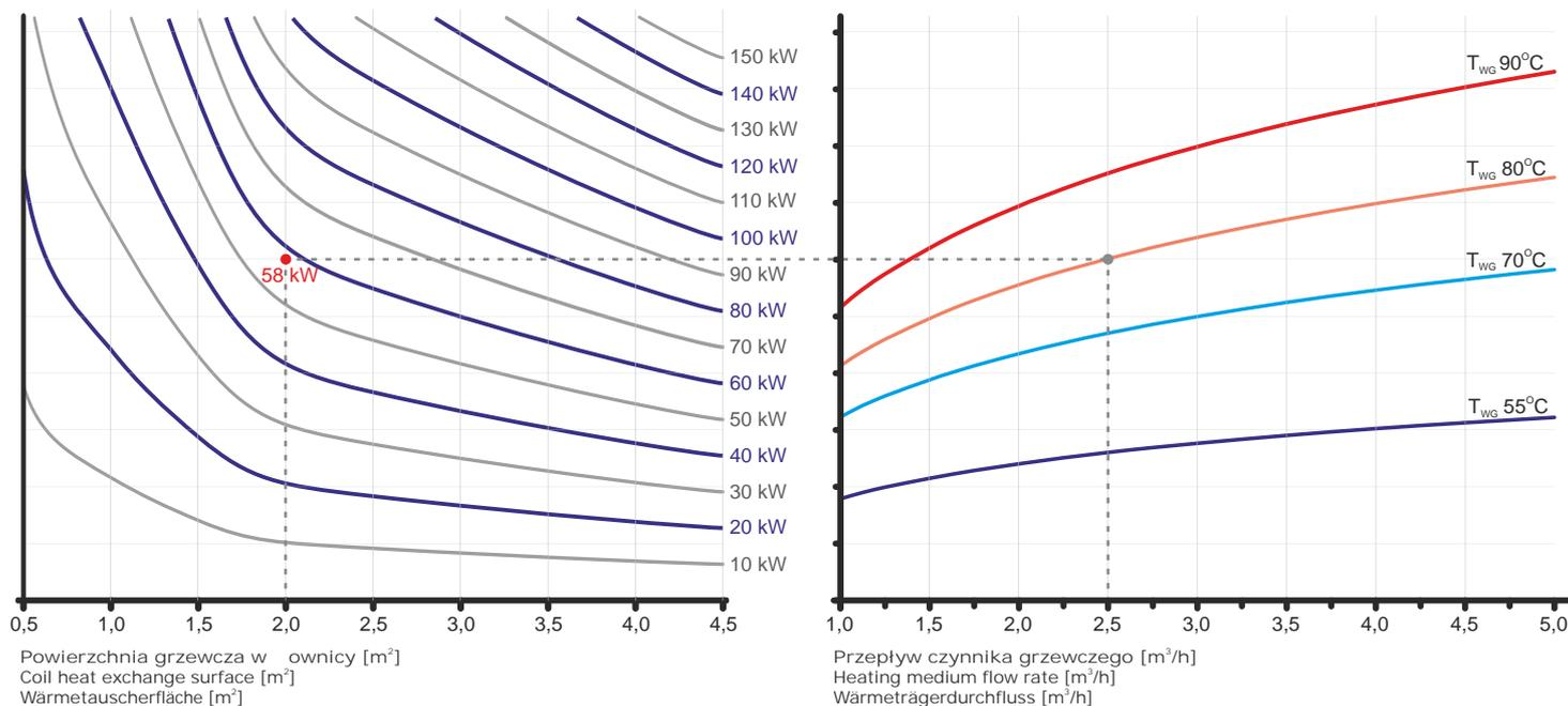
[ $T_{wg}$ ] - Temperatura wody grzewczej / [ $T_{wg}$ ] - Temperature of heating water / [ $T_{wg}$ ] - Heizwassertemperatur.
